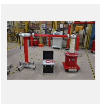
Specialized Partial Discharge Testing
